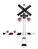
**CROSSING GATES** often have flashing red lights and bells to warn pedestrians and drivers that a train is approaching. Always stop when lights are flashing and never go around or under a gate. Look and listen, these signals will alert you when it is safe to cross.
